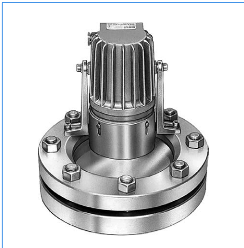
Safe area type KL PowerLED Sch B, 24 V AC / DC, 7 W, with anti-dazzle shield "B", on circular sightglass to DIN 28120, DN 150, PN 10, in version "view and light through one sightglass".
