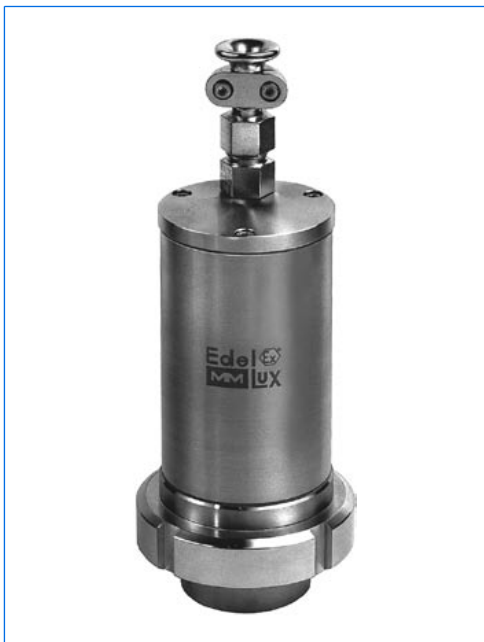
Sightglass light fitting type EdelEx d LED R50 K1, ca. 2 W, 24 V, Ex d IIC T6, Ex tD A21 IP65 T80°C, Ex II 2 G + D, with intermediate flange collar fixation "R", mounted onto a screwed sightglass similar to DIN 11851, PN 6, DN 50.
