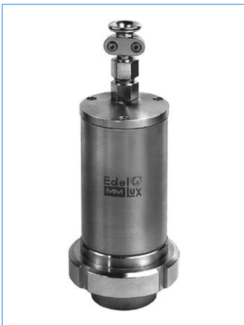
Sightglass light fitting type EdelEx d LED R50 K1, 2 W, 24 V AC/DC, Ex d IIC T6 Gb, Ex t IIIC T80°C Db, IP65/67, Ex II 2 G + D, with intermediate flange collar fixation "R", mounted onto a screwed sightglass similar to DIN 11851, PN 6, DN 50.
